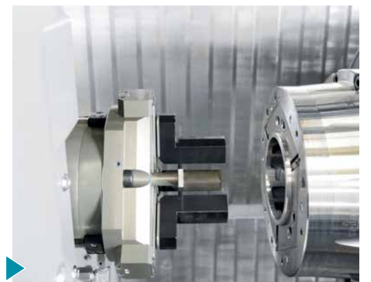
3-axis workpiece handling for flange parts
