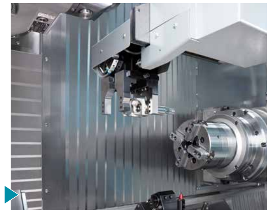
Removal of finished parts (or feeding) using a workpiece-specific gripper for shaft or flange parts
