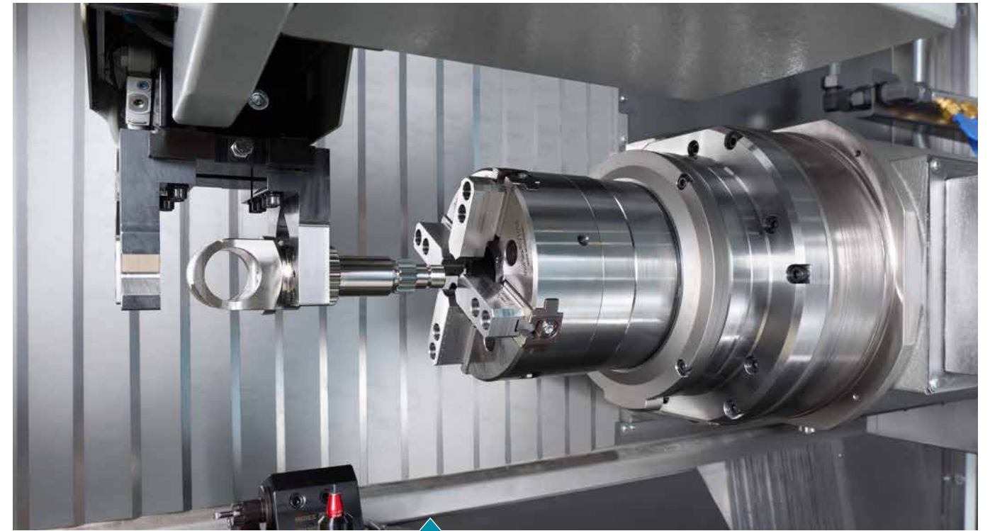
Removal of finished parts (or feeding) using a workpiece-specific gripper for shaft or flange parts
